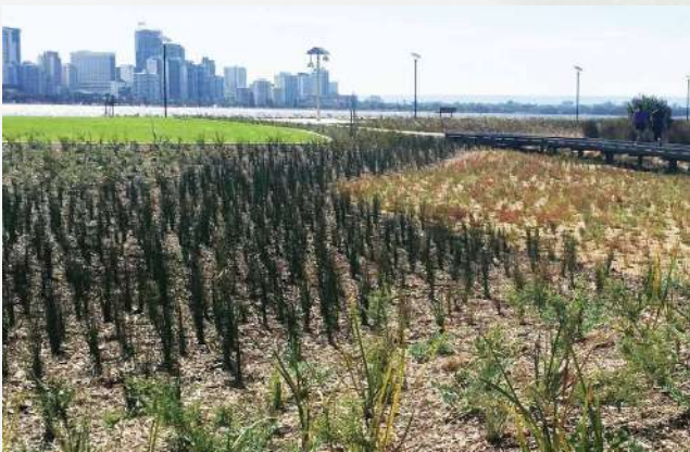
SWALES / RAIN AND BIO-FILTRATION GARDENS
