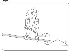
Begin by marking out the desired line for your edging using a suitable survey marking product.
