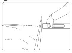
For straight sections use a builder's line set at the finished height of the edging.
