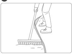
Once the edging is secure, use a rake or shovel to backfill the trench with the soil or material you initially removed.
