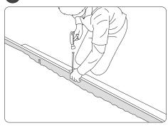
In conjunction with leveling the edging in the previous step, insert the supplied braces along the edging length.
