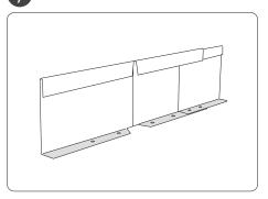
Prefabricated corner pieces are available for all sizes. They are supplied flat so they can be bent to any angle onsite by hand.
