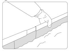
Where two pieces of edging meet, use joiners to connect the section securely.
