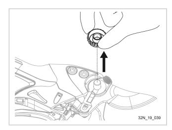
6. Remove the shaft from the blade
