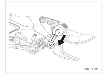
8. Remove the adjustment washer
