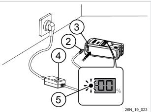
Connect the charging cord (2) to the battery's charging connector (3). The charger indicator (4) lights up green, and the battery indicator (5) flashes orange.
