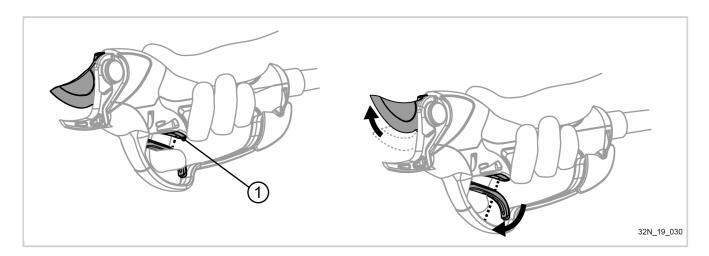
The blade stays half-open as long as the optical system (1) detects your finger on the trigger. When your finger releases the trigger, the optical system tells the blade to open fully.
