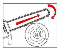
• When the guide plate is used for a bottom-up cut, the pushing direction of the chainsaw is towards the operator.
